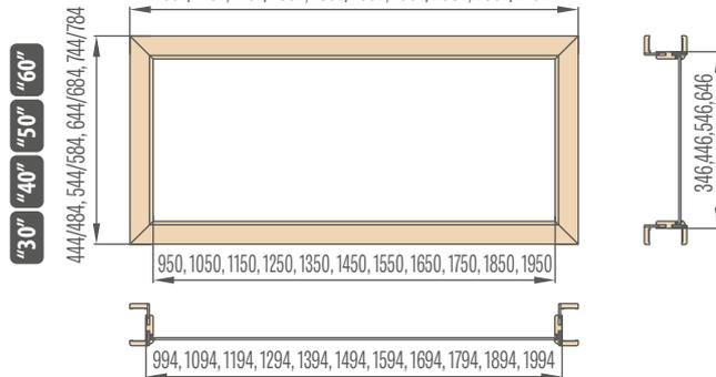
Calculation scheme for the wall opening height
