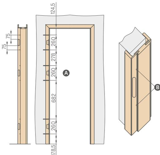
**A** Drill holes for metal screws of min length 80 mm x  $\varnothing$ 6 mm
