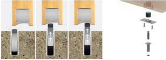
We assemble the magnetic door stop in a special place milled for this purpose on our own. Product delivered as a separate assortment.
