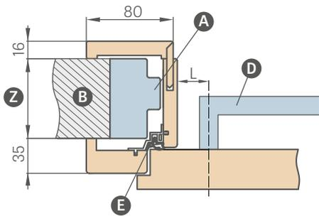
L – distance between the handle centre line and the frame strip edge
