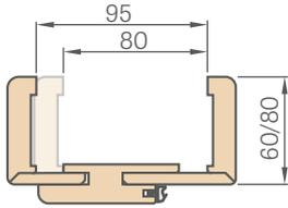
The square tongue is to be trimmed by a customer to required size, for door frames within 80-95mm range
