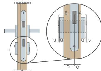
Example of calculating the lock core size for the flush and panelled doors (40mm) with the escutcheon thickness of G = 7 mm
