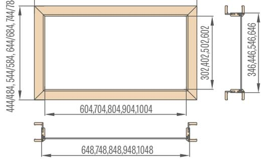
Top lights for adjustable door frame in rebated double doors architrave 6 cm / architrave 8 cm
