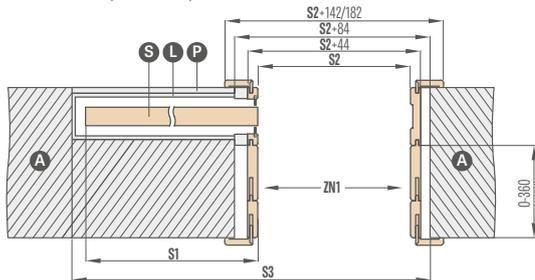
The drawing shows a one-sided basic in-wall installation ZN1.
