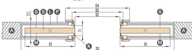
Only for use with flush doors which are supplied with a glass frame.
