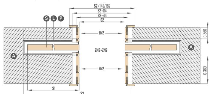
The drawing shows double-sided the basic in-wall installation ZN2 + ZN2.
